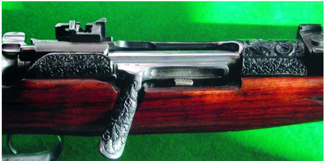
**Above: The Cogswell & Harrison Certus rifle with the action open, showing the bolt on its sliding carrier. Lower: German Steyr Daimler Puch rifle built on a Mannlicher-Schoenauer action, the telescopic sight mount set on the side of the receiver.**
